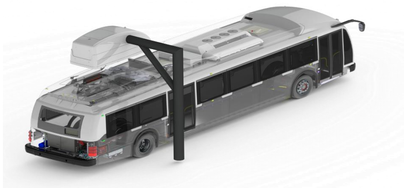
Battery Electric Bus Depicted with On Route Fast Charging Stand
