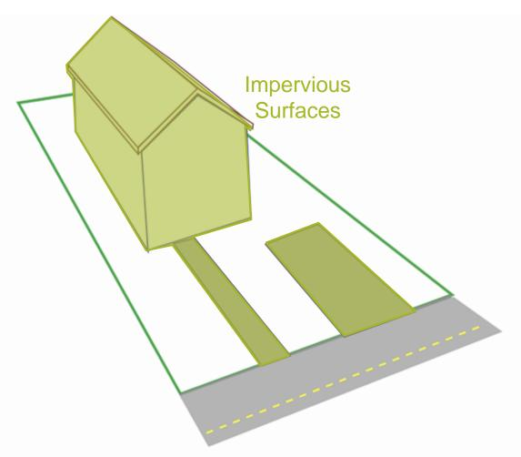
Impervious Surface Ratio determines the amount of land that can be covered with material that can't absorb water (impervious). It's calculated by multiplying the lot size by the ratio set by the Land Use Management Ordinance (LUMO).
