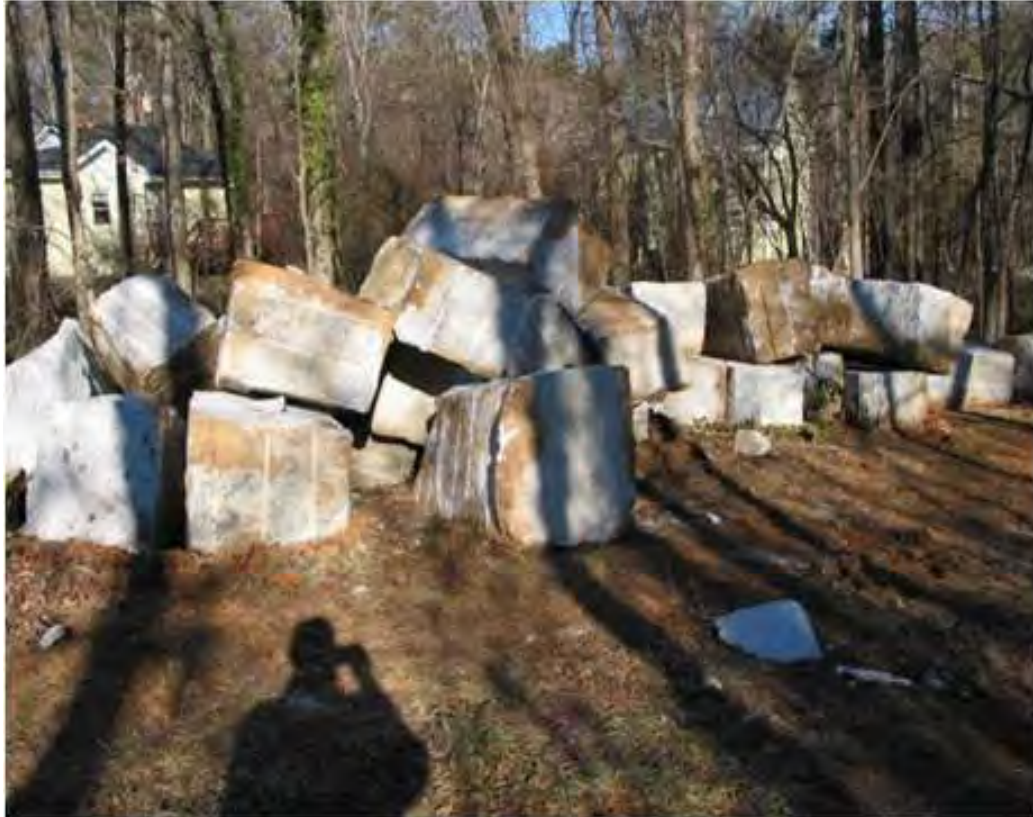
The giant(8'x4'x4') rocks used to create the step-pools
