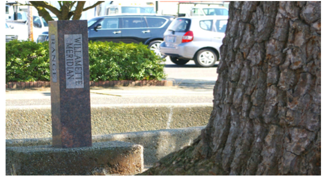
Survey monument in the Fountain Plaza Park.
