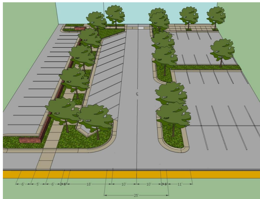
45 ° Angled parking - parking bays
