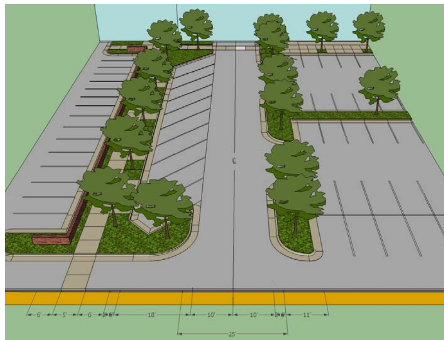
45 ° Angled parking - parking bays
