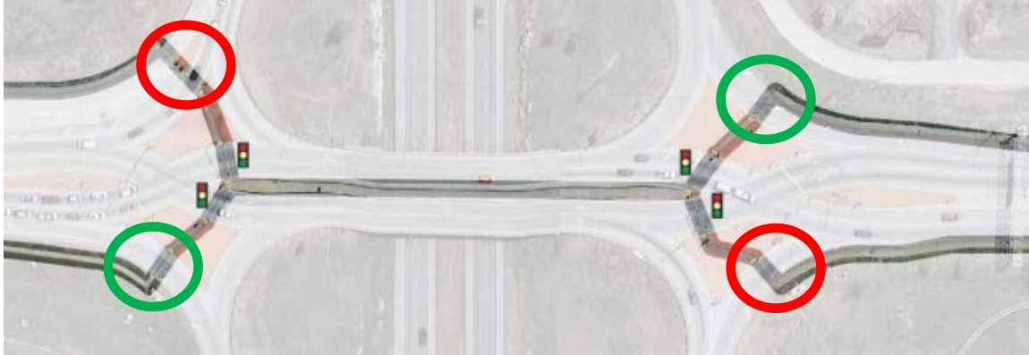
Figure 2 - DDI in Springfield, MO. Source FHWA DDI Informational Guide. Accelerating free flow ramps are circled green, decelerating ramps are circled red.
