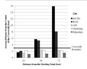
*Figure 3.* Average linear deviation from the center of the crosswalk by cue condition and crossing length.
