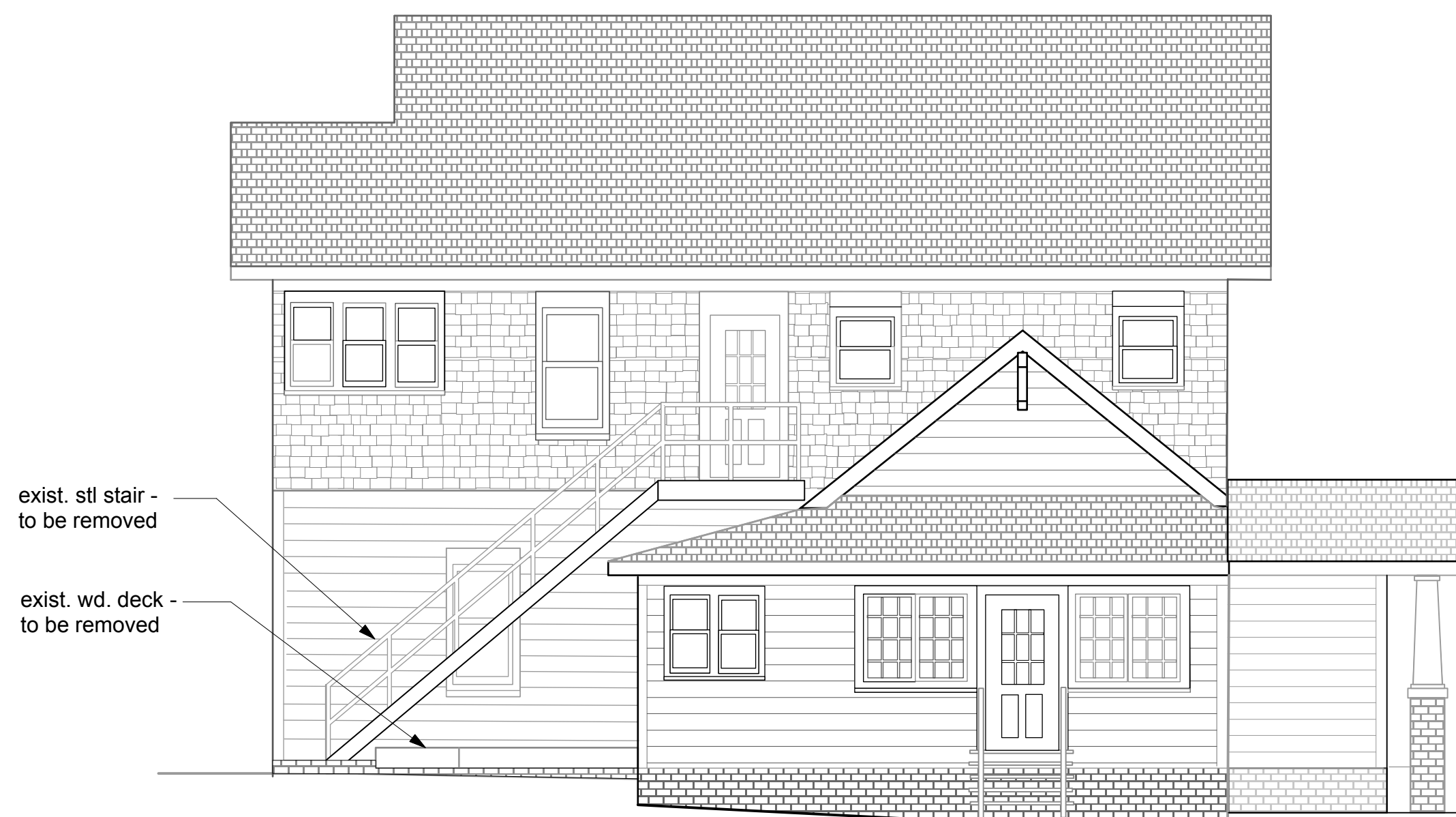
East Elevation, Existing- 3/16"
