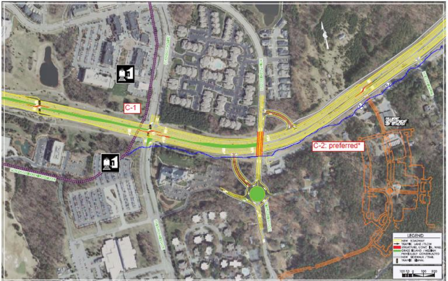
Figure 6-16: Recommended Barbies Chapel Grade Separation Design.
