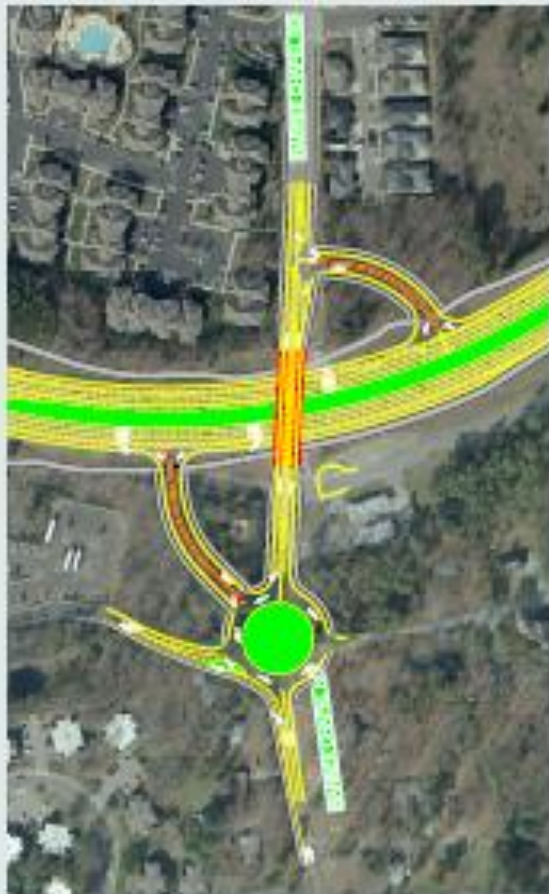
Figure 6-16: Recommended Barbies Chapel Grade Separation Design.
