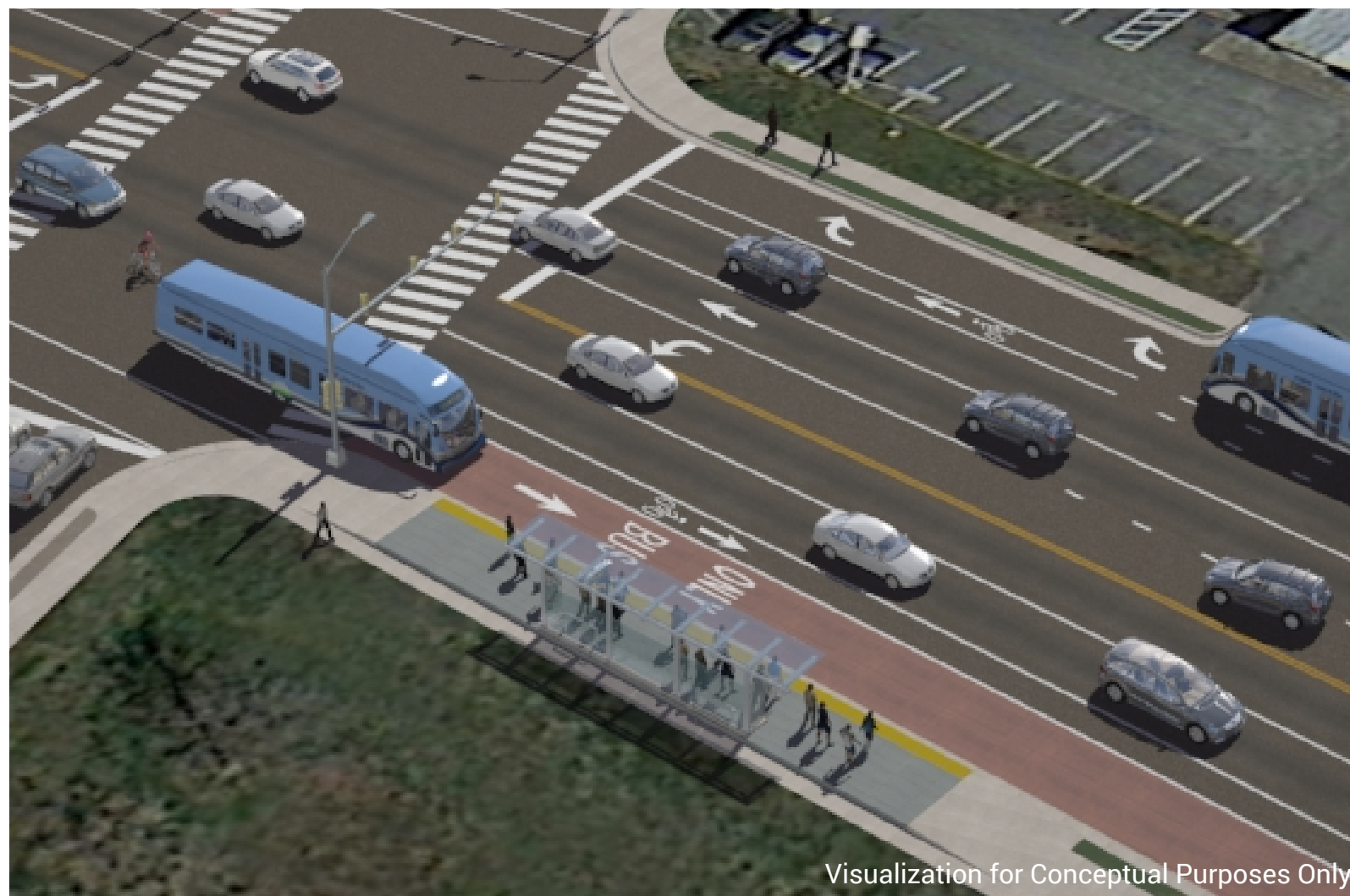
Dedicated Curb Lane - Construct a New Lane
