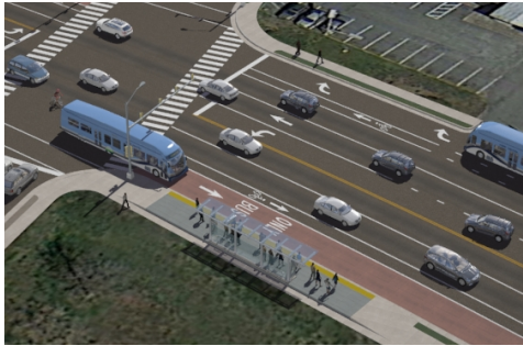
Dedicated Curb Lane - Construct a New Lane
