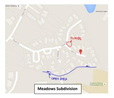
Clover Dr. and Lark Circle intersection is vulnerable to flooding after debris accumulates in culvert. Open swale at southern side of Meadows Subdivision is not being maintained. This appears to be a private ditch. No insurable structures are affected from this flooding.
