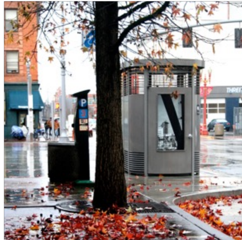
The Portland Loo is a simple, high-quality sidewalk toilet that illustrates design criteria of maximum function in minimum space, safety, cost effectiveness, accessibility, availability, attractiveness and ease of maintenance.
