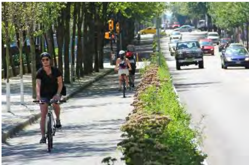
Example of cycle track using planter buffer in Vancouver, BC >
