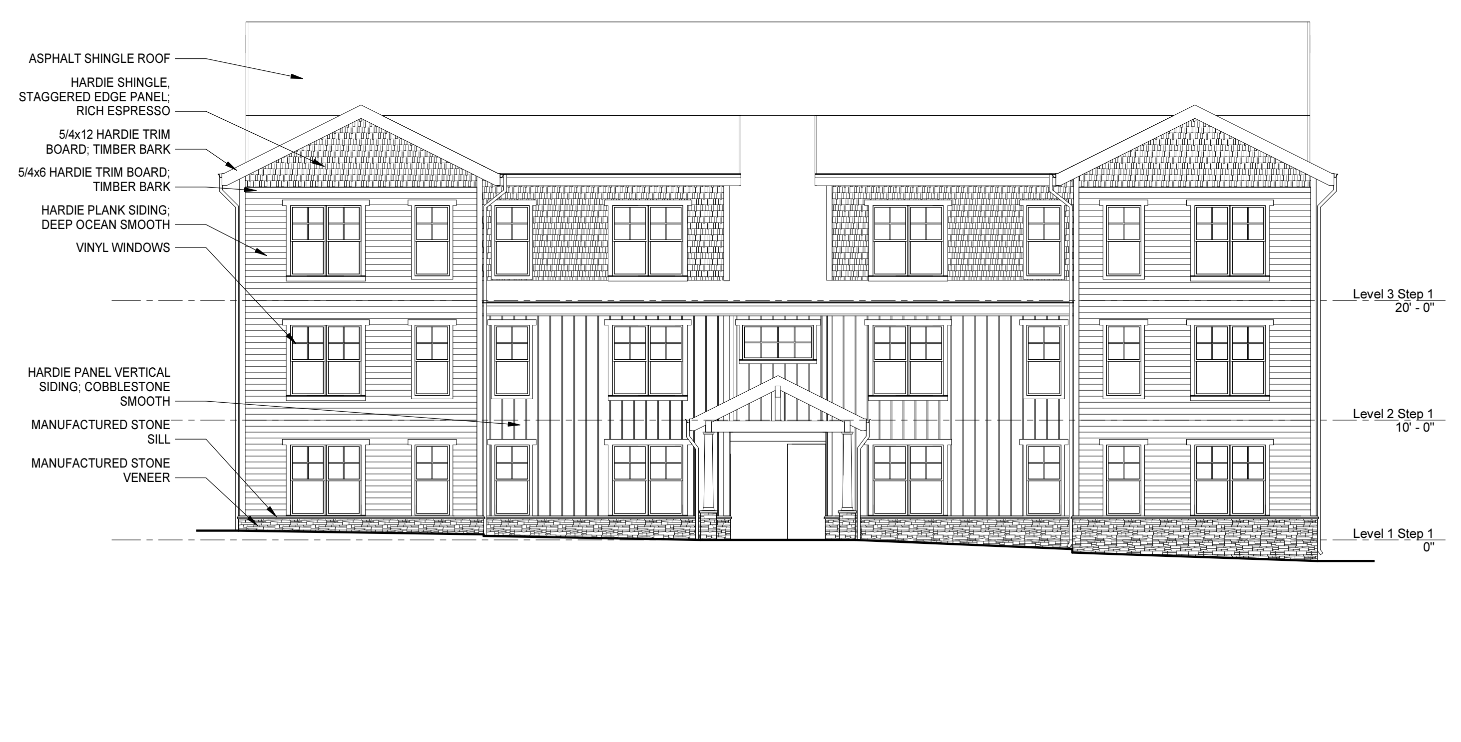
1 SOUTH ELEVATION - BUILDING B 1/8" = 1'-0"
