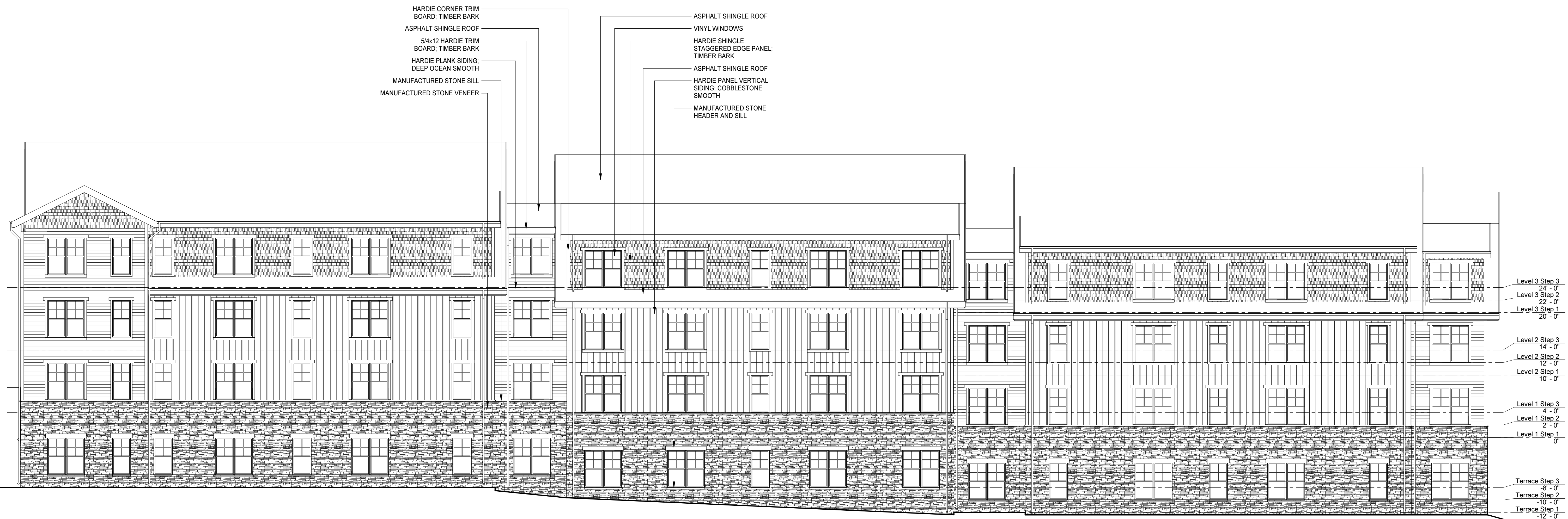
1 NORTH ELEVATION - BUILDING A 1/8" = 1'-0"
