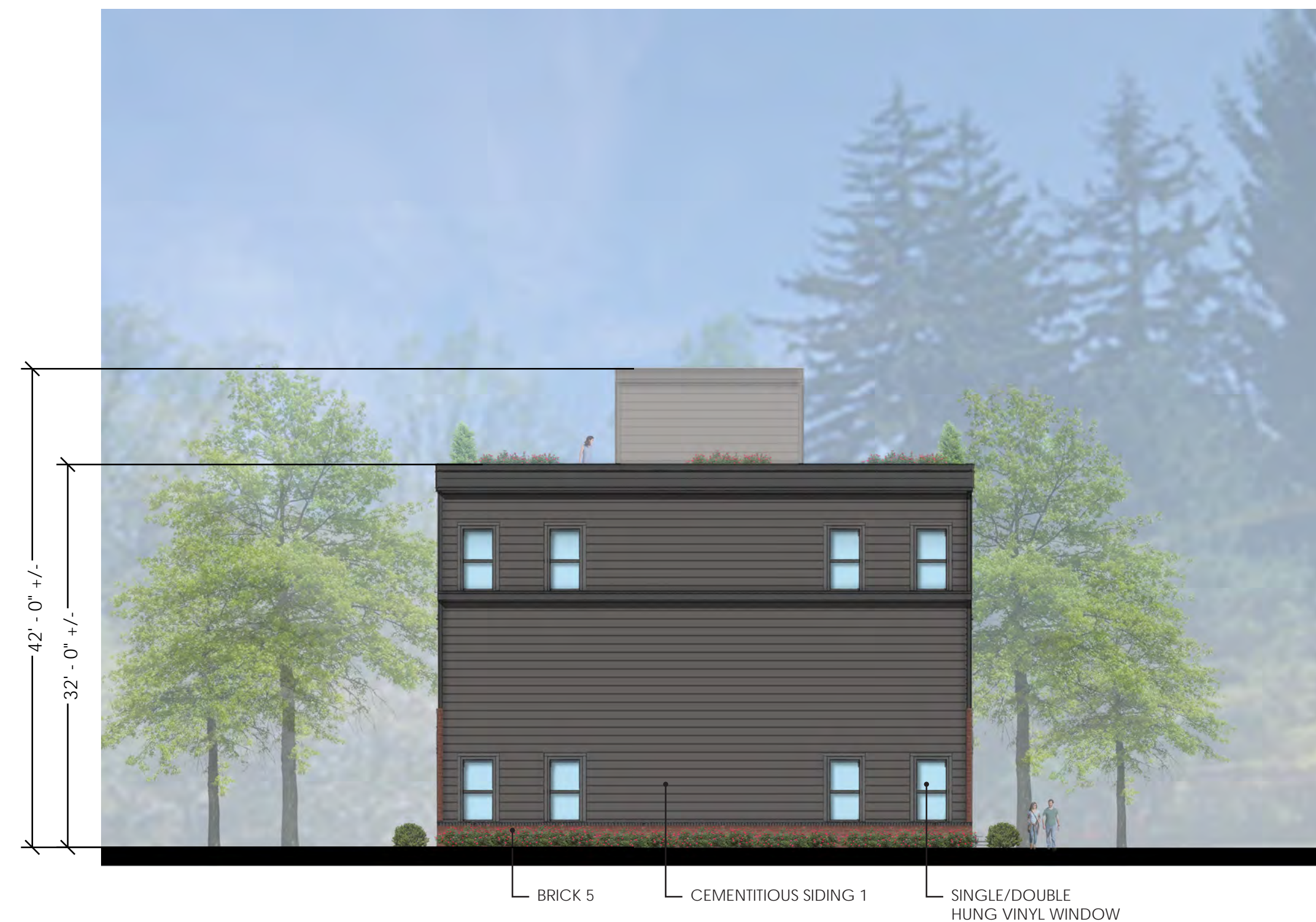
2 - SIDE ELEVATION SCALE: 3/32" = 1'-0"
