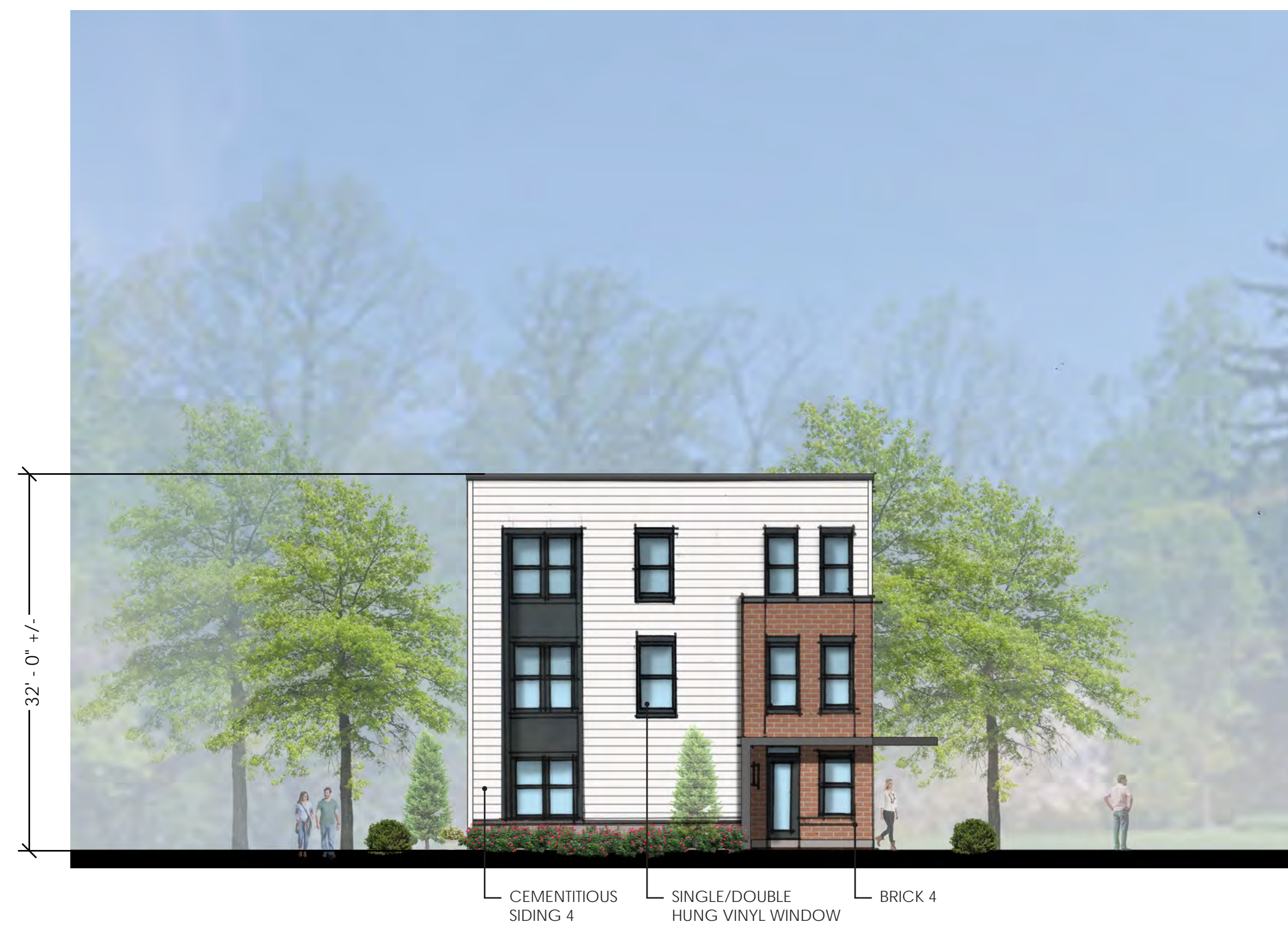
2 - SIDE ELEVATION SCALE: 3/32" = 1'-0"
