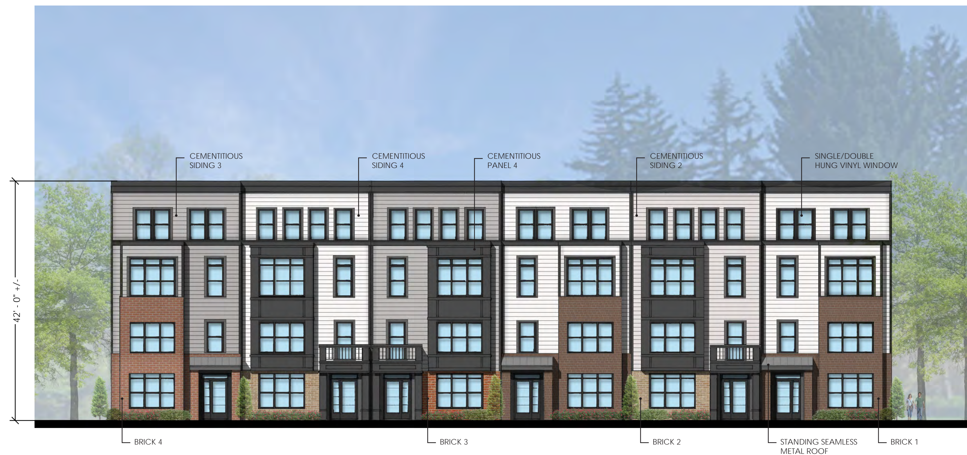
1 - FRONT ELEVATION SCALE: 3/32" = 1'-0"
