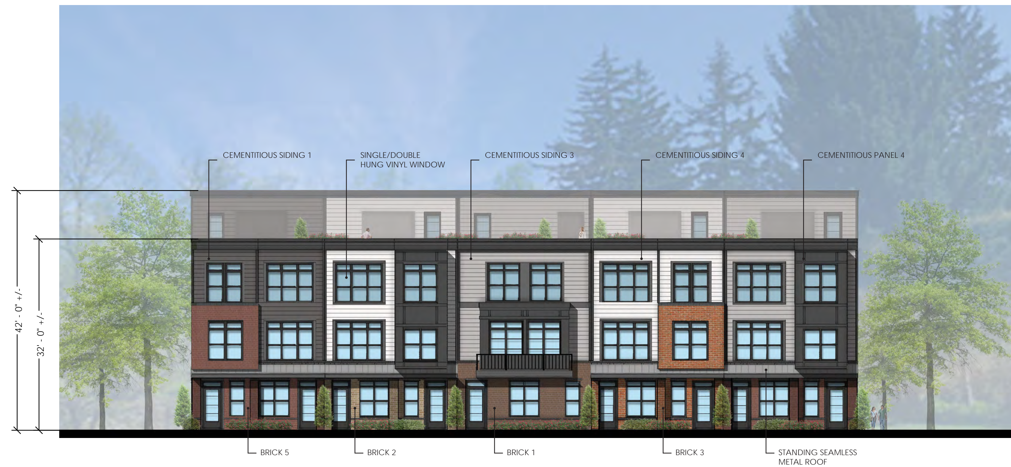
1 - FRONT ELEVATION SCALE: 3/32" = 1'-0"
