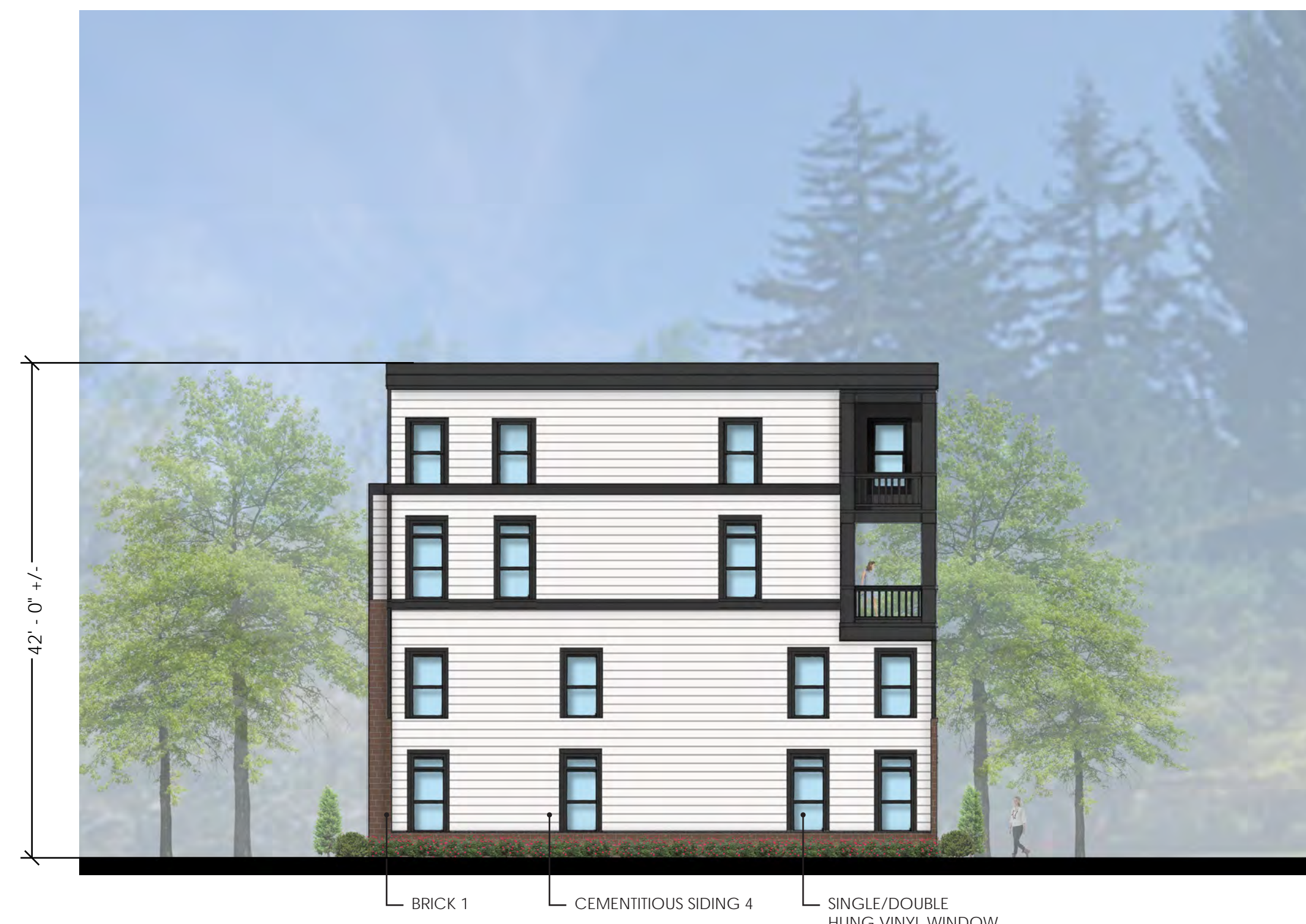
2 - SIDE ELEVATION SCALE: 3/32" = 1'-0"
