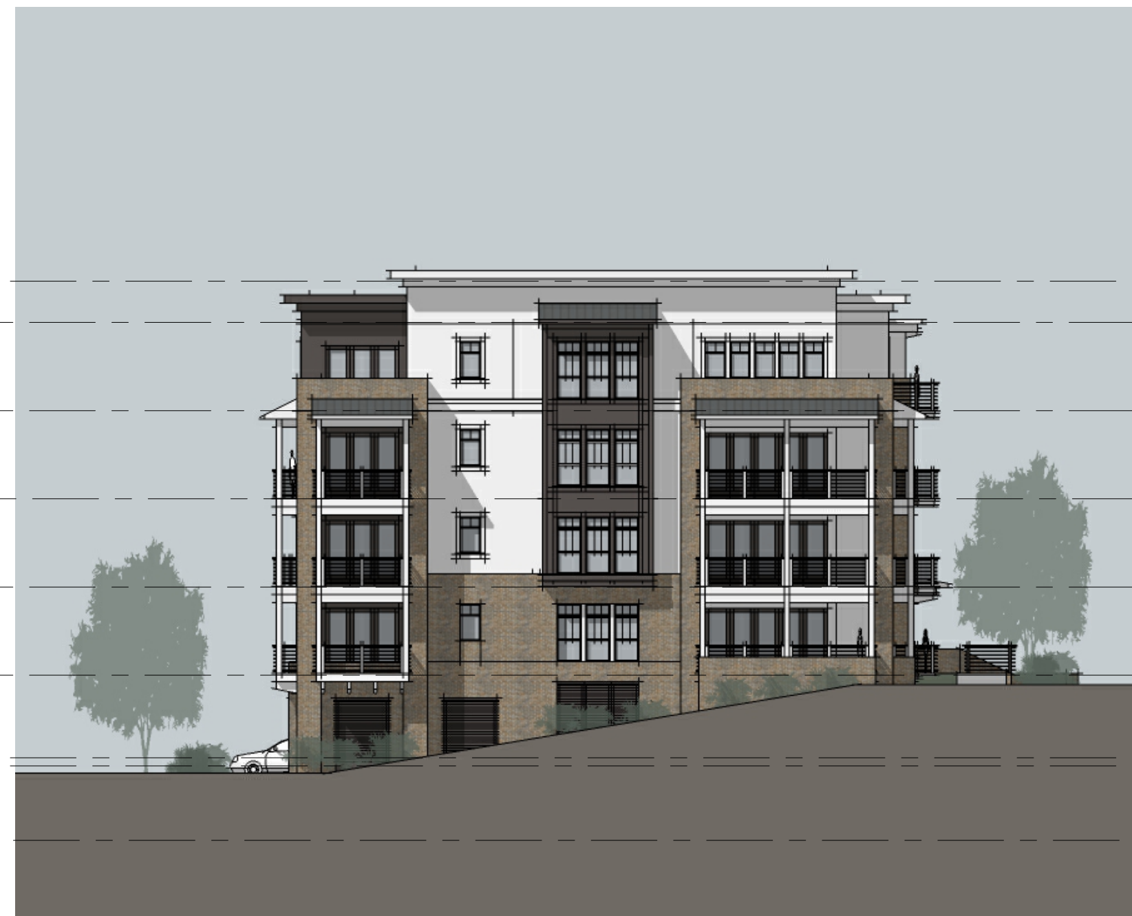
Typical "Short" Condominium - Side Elevation 1/16" = 1'-0"
