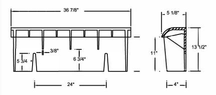
STORMDRAIN CURB INLET HOOD FOR INSTALLATION ON STATE STREETS. AND INSTALLATIONS UNDER THE JURISDICTION OF THE NORTH CAROLINA DEPARTMENT OF TRANSPORTATION AND SHALL COMPLY WITH ASTM A48 CL35. IT SHALL BE A HEAVY DUTY TRAFFIC BEARING GRATE WITH AN APPROXIMATE TOTAL WEIGHT OF 575 LBS. (INCLUDES WEIGHT OF GRATE, FRAME & HOOD).
