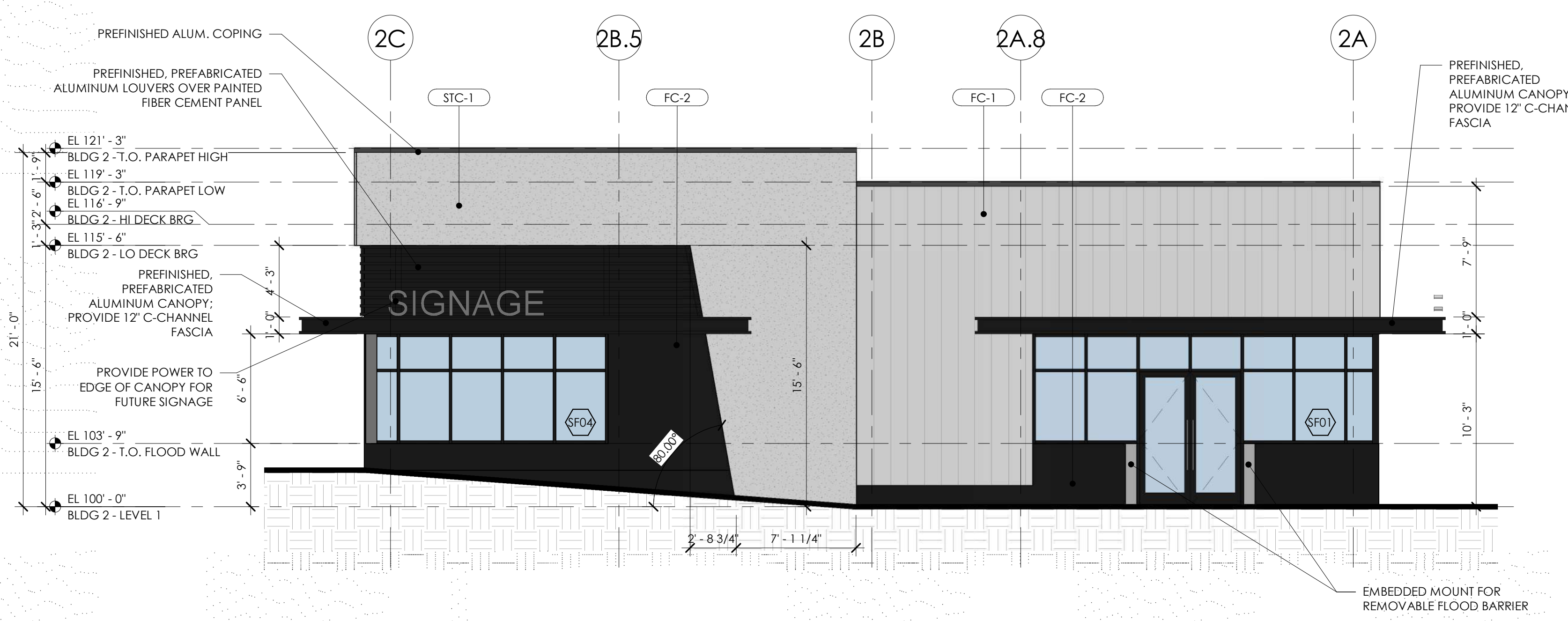
BLDG 2 - WEST ELEVATION A4.02 SCALE: 3/16" = 1'-0"
