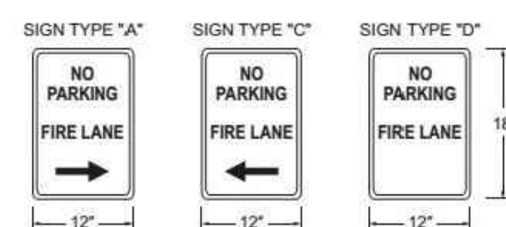
FIGURE D103.6 FIRE LANE SIGNS
