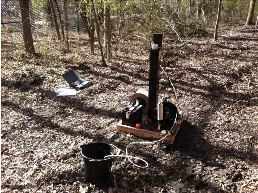
View of water purging activities at MW-4
