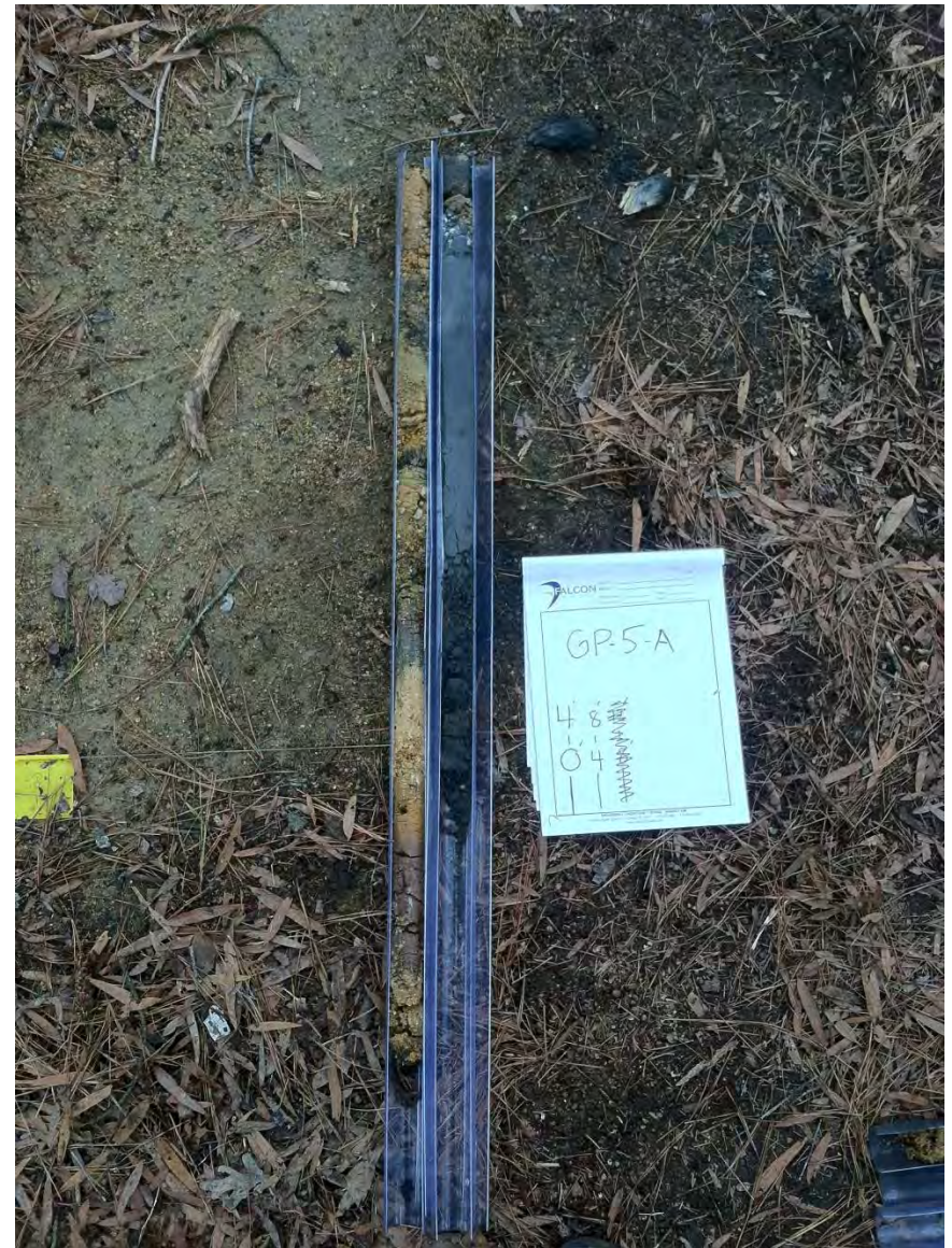
GP-5-A soil profile (shallow refusal)
