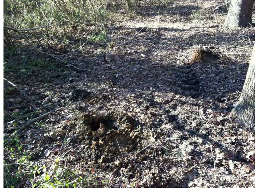
Two auger holes having refusal for MW-4
