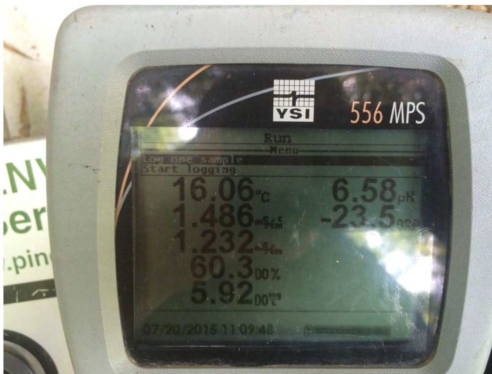
YSI Instrument Reading – Between 1 st and 2 nd Purge – MW-3A
