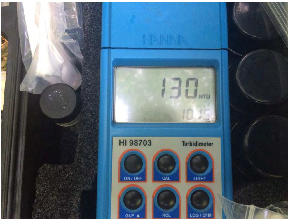
First Purge Turbidity Reading – MW-3A
