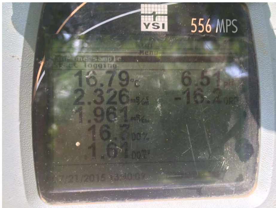
YSI Instrument Reading – 7 th Purge – MW-3A
