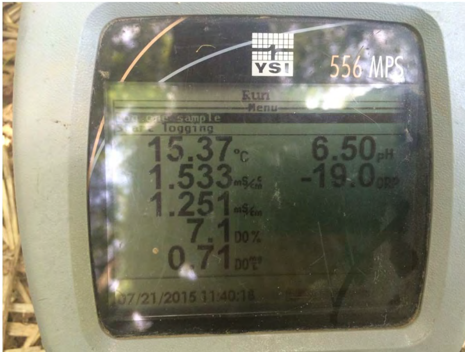
YSI Instrument Reading – 6 th Purge – MW-3A 7/21/2015
