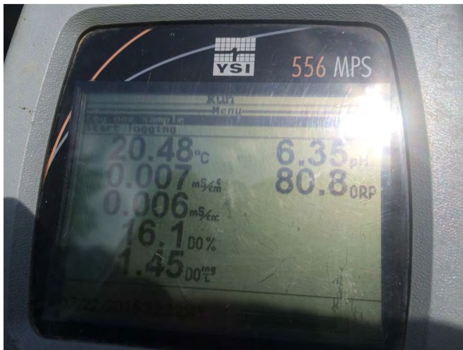
YSI Instrument Reading – 13 th Purge – Well-1
