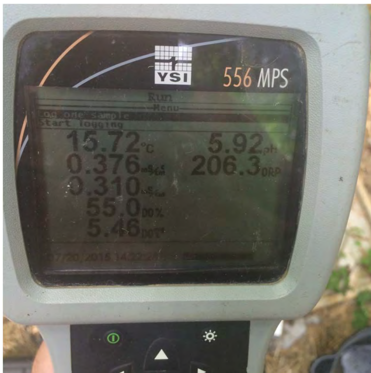
YSI Instrument Reading – 4 th Purge – MW-4A
