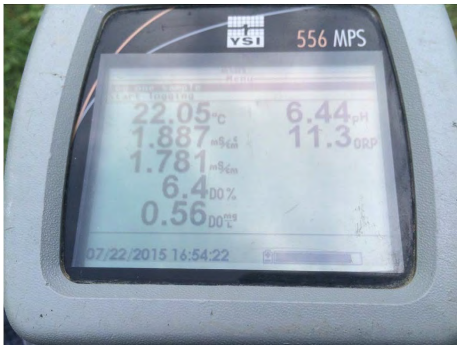
YSI Instrument Reading – 17 th Purge – Well-1
