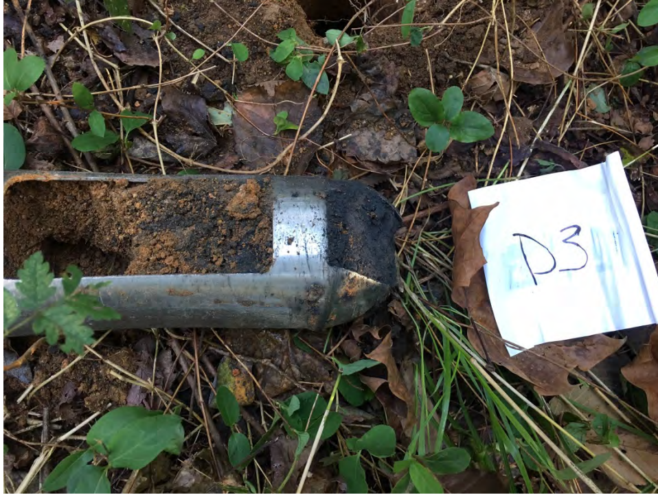
Photograph 1: Example of CCP in stainless steel hand auger from CCP Evaluation Boring D3.
