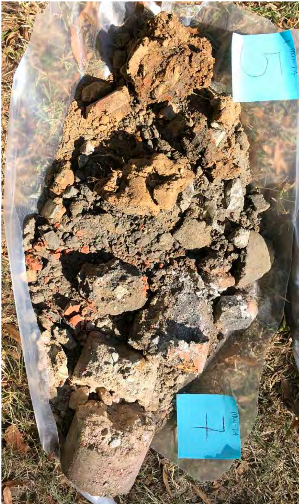
Photograph 1: 5-7 ft bgs (from top to bottom of the page) in MW-1A
